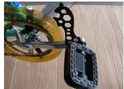
Please note you need to screw the right pedal clockwise into the crank eye, and screw the left pedal anti-clockwise into the crank eye. If it does not turn easily do not force it and double check that you have chosen the correct pedal doing in a correct way. *Forcing the wrong pedal going in will damage the thread on your pedal and crank arm.*
