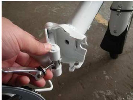
When unfolding, swing your frame together. Make sure the quick release bolt snaps into the frame folding box.
