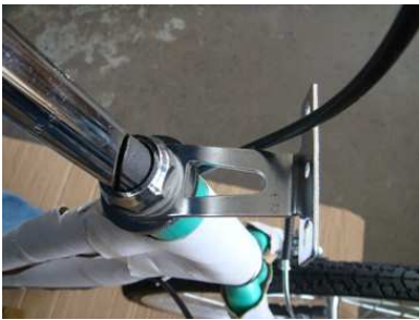
Insert the stem into head tube
