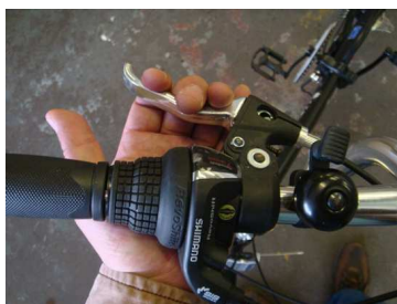
D: Rotate the lever and adjust the angle
