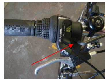
D: Rotate the lever and adjust the angle
