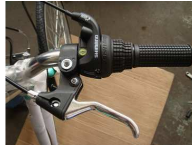
B: Insert the cable into the hole
