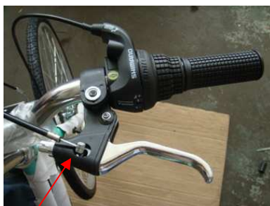
B: Insert the cable into the hole
